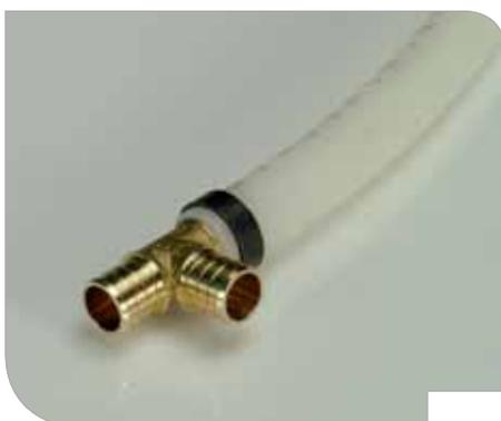
3. Insert the fitting into the pipe up to the fitting shoulder. Position the crimp ring 3-6 mm from the end of the tube.
