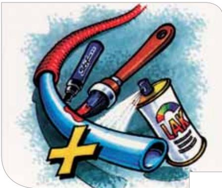
8. Ensure contact with products containing solvents, such as sprays is avoided.
