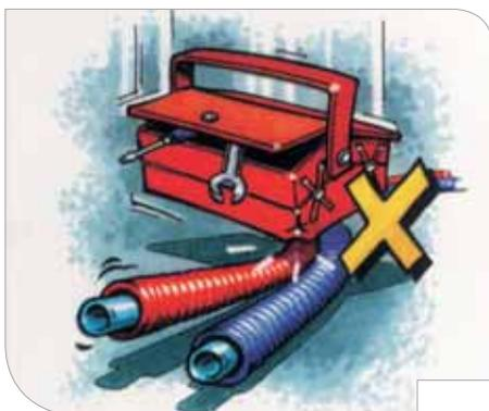
3. Pipe must be protected against mechanical damage.
