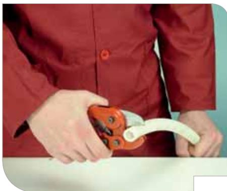
1. After having cut the pipe being sure that you have a square burr-free cut. An uneven cut may cause an improper connection.
