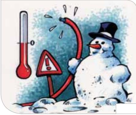
7. If there is any risk of freezing, drain the pipe or use an anti-freeze solution.
