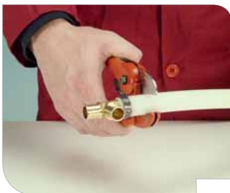
Don't try to save time by re-crimping a crimp that does not gauge properly. The fitting must be cut out and re-placed.
