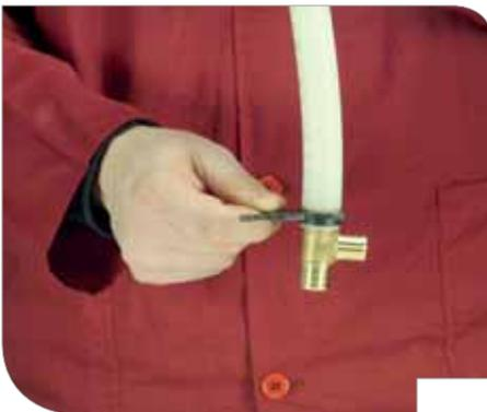
Always place the gauge opening on the crimp ring at a 90° angle for an accurate check.
