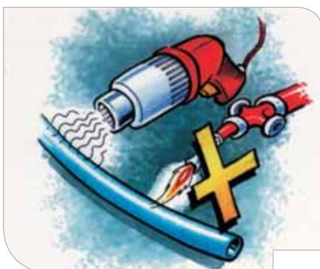
6. For bending the pipe with heat, or repairing it, heat the pipe till it becomes transparent (max. 140°C) and use hot air only (PEX only). Do not allow the pipe to come into direct contact with flames.
